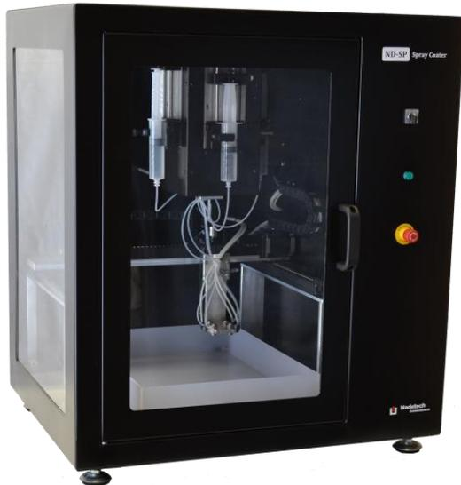
Nadetch ND-SP Precision Spray Coater is a completely automatized equipment for thin film deposition via spray coating, where uniformity and small drop sizes are required. Its design and programmable software allows to control and automatize every deposition parameter with high precision and reproducibility. ND-SP Precision Spray Coater is used to obtain homogeneous coatings with one or multiple layers.
